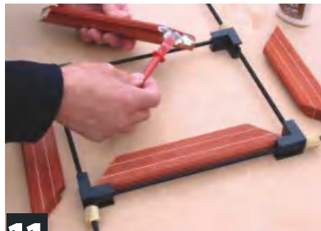
11 Set out a Veritas cramp ready for the frame. Apply PVA glue to the mitres and position the pieces. Firmly tighten each corner adjuster
